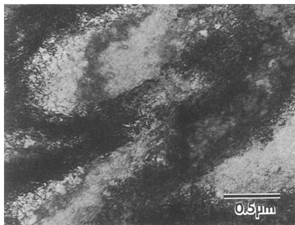
Figure 5 Transmission electron micrograph of the Cu-7% Ni-3% Al alloy aged at 500^\circ\text{C} for 10^3 s.
