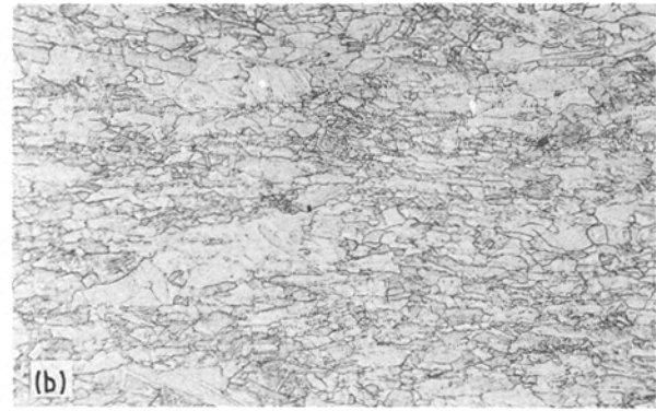
Figure 11 Optical micrographs of Cu–Ni–Al alloy aged at 680 °C for 2 h. (a) Cu–4% Ni–3% Al, (b) Cu–5.5% Ni–3% Al, (c) Cu–7% Ni–3% Al.
